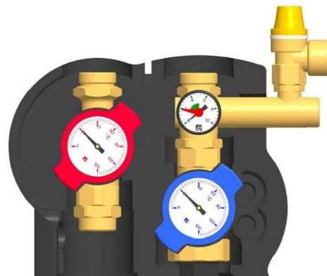
Turn thermometers 45° to open flow check valves during initial flush and fill.
